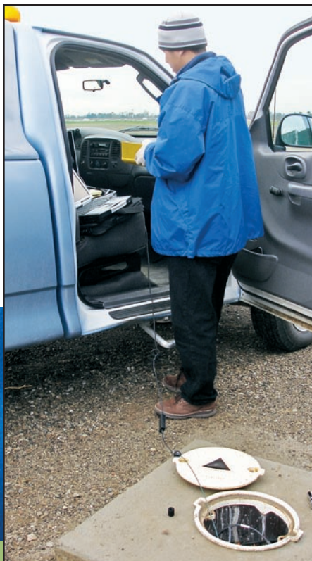
Downloading pressure transducer data from a monitoring well.
